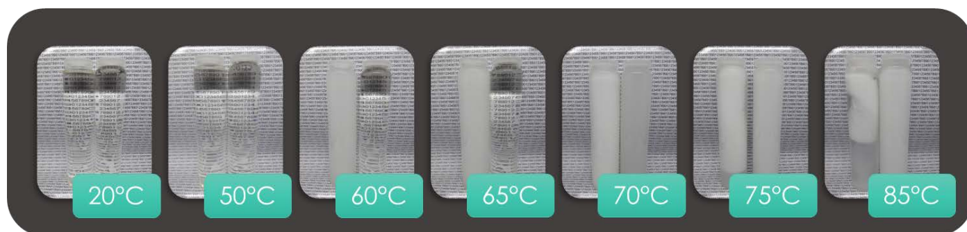
figure 4: thermal gelling effect of 2% aqueous solutions of E (left) and K(right) -type binder
